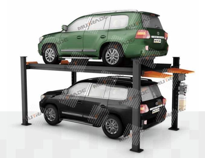
Specially developed for heavy-duty parking purpose based on traditional 4 post car lift, offering parking capacity 3600kg for heavy SUV, MPV, pickup, etc. Hydro-Park 2236 has rated lifting height of 1800mm, while Hydro-Park 2336 is 2100mm. Two parking spaces are offered above each other by each unit. They can also be used as car lift by removing the patented movable cover plates at platform center. User can operate by the panel mounted on front post.
