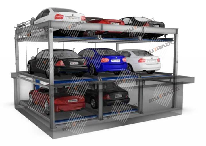
The system is semi-automatic puzzle parking type, one of the most space-saving system that parks three cars on top of each other. One level is in pit and another two on above, the middle level is for access. The user slides his IC card or inputs the space number on operation panel to shift spaces vertically or horizontally and then move his space to entry level automatically. Safety gate is optional to protect cars from theft or sabotage.
