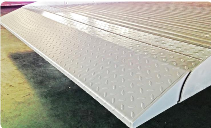
Powder coating is applied as a free-flowing, dry powder. It is typically applied electrostatically and is then cured under heat to allow it to flow and form a "skin". It is usually used to create a hard finish that is tougher than conventional paint.
